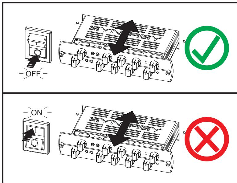
You should always turn OFF your amplifier or pre-amplifier before installing or removing a module. Failure to do so can cause damage to your preamp module or amplifier.
